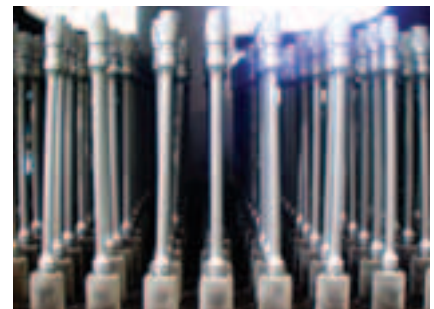
Fig. 6. Mechanical masking of torsion bars during ion nitriding; bars are positioned in the steel bushings, which serve as locators, as well as mechanical masks.
